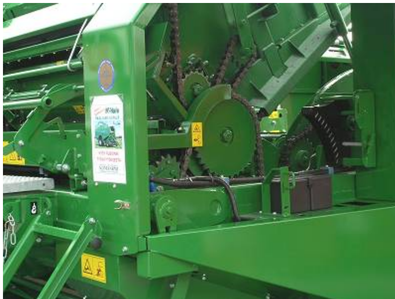
Chains of a roller baler, safety signs in place - Courtesy of FIOH
