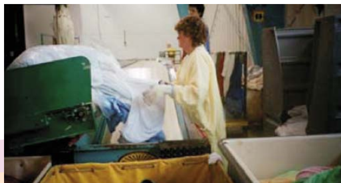
Figure 2: Feed conveyer after modification, showing an extended conveyer and the use of plastic linen bags
