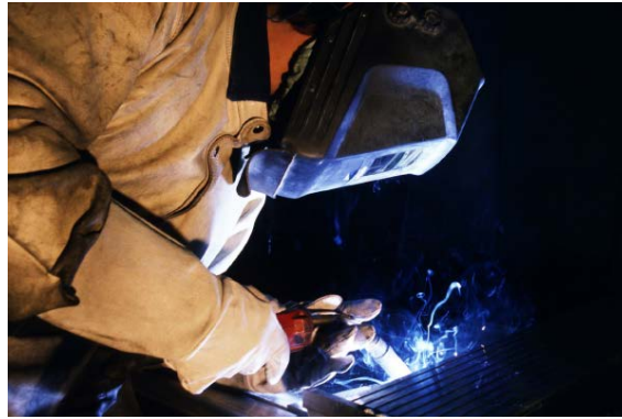
Figure 2: Welding fumes contain irritating gases and vapours as well as ultrafine particles, HVBG/Senn
