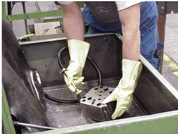
Figure 4: Cleaning metal with a vegetable oil-based ester, KOOP
