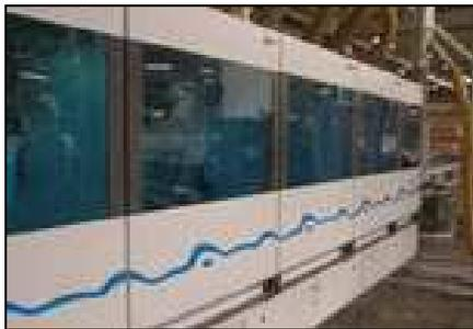
**Figure 5. Some machine tools that produce a lot of dust are now enclosed in special chambers**
