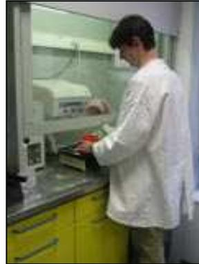
In the same way, the operation of filling bronze moulds with resin and compressing it, which causes the emission of noxious, flammable methyl methacrylate vapours, is now performed under a ventilated hood.
