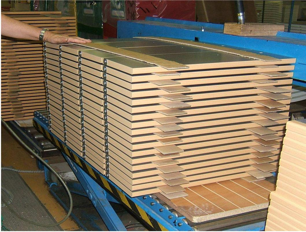
Figure 1 Use of a scissor lifter
