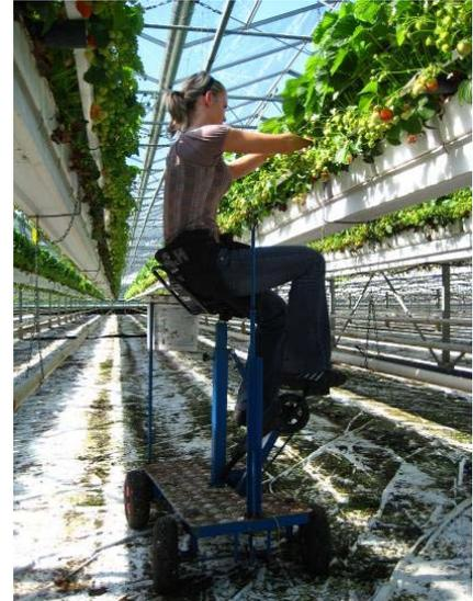
Left: the crop cultivation bicycle. The handle that steers the front wheels is left to the seat, a holder to carry a bucket is right to it. Right: riding the bicycle while pulling blossoms through.
