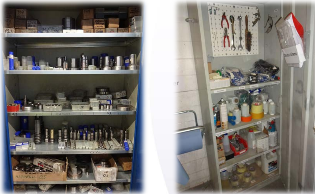
Figure 4: An example of two new storage cupboards for equipment, installed after the implementation of the 5S system (photo: Saku Metall AS).
