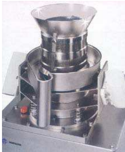
Figure 1: Mixer for obtaining hydrogels based on zinc oxide and titanium dioxide doped with silver
