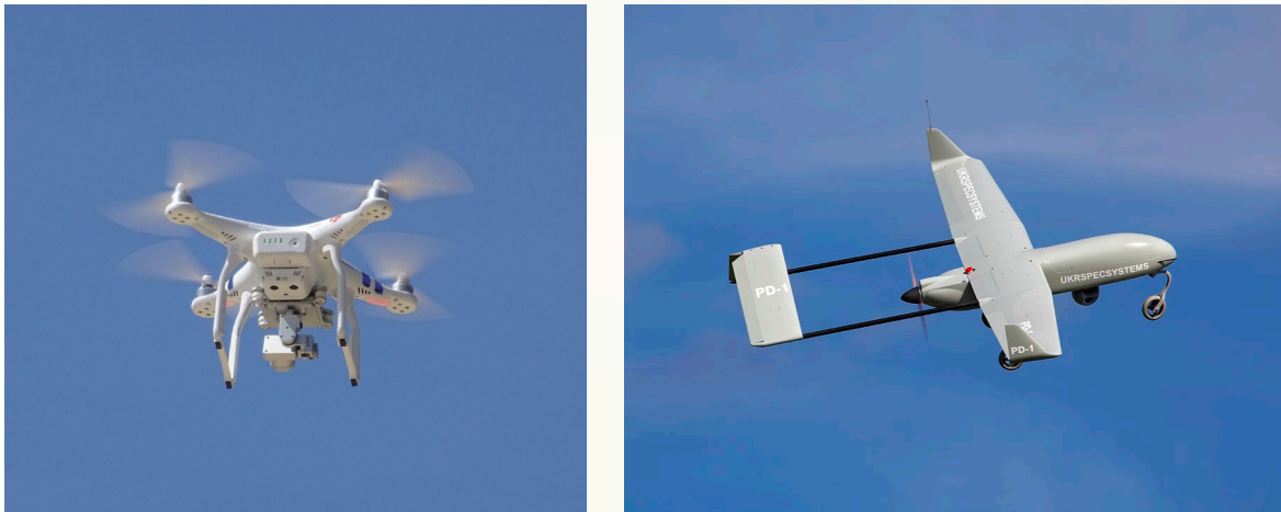
Figure 1: UAV typologies. A four-rotor drone on the left (the load is visible in the underside of the drone – www.publicdomainpictures.net ). A fixed-wing UAV is shown in the right image ( People's Drone PD-1 by DoroshenkoE, Wikimedia Commons, licenced under CC-BY 4.0 ).
