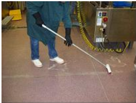
Figure 3. Use of scrapers to remove major debris
