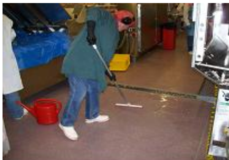
Figure 4. The residue of debris, fat and grease is led to a drain
