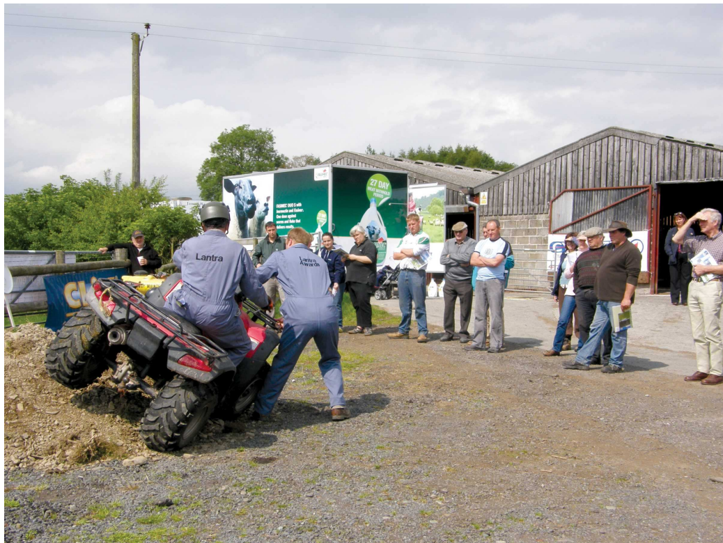
Figure 3: Lantra trainers demonstrate how weight distribution affects ATV's stability
