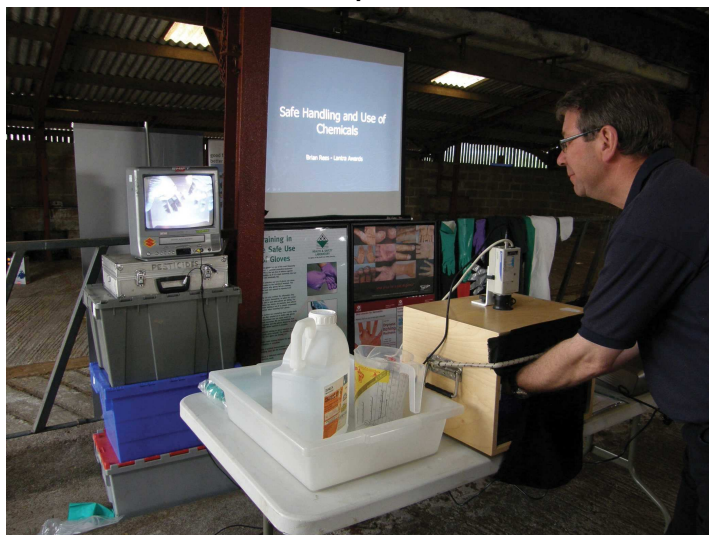
Figure 1: By using a light box, HSE advisors show how chemical contamination may be present on hands despite it not being visible to the naked eye, and can show how different handling techniques and appropriate personal protective equipment can minimise exposure.
