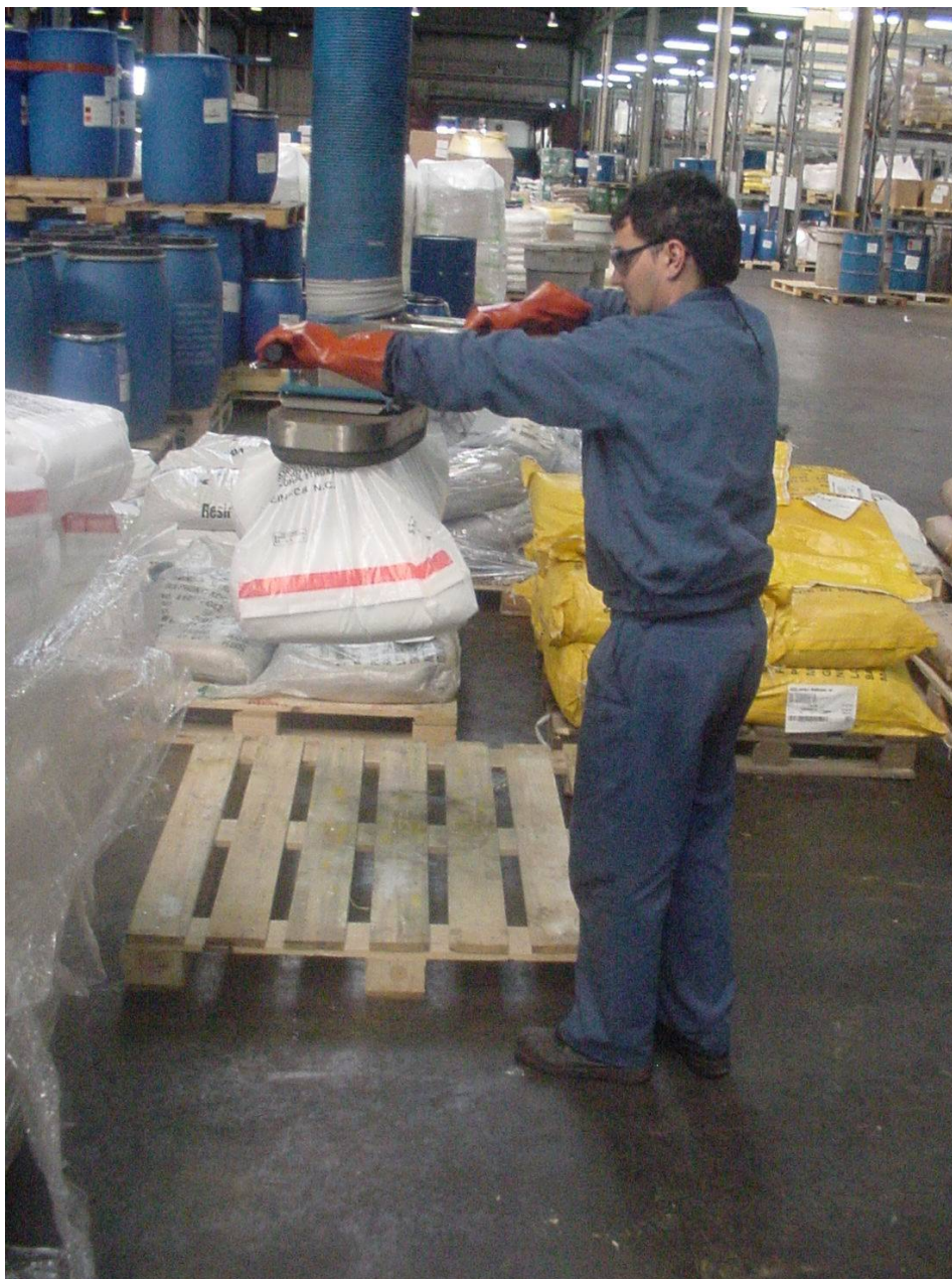
Figure 6. Vacuum lifting system in operation
