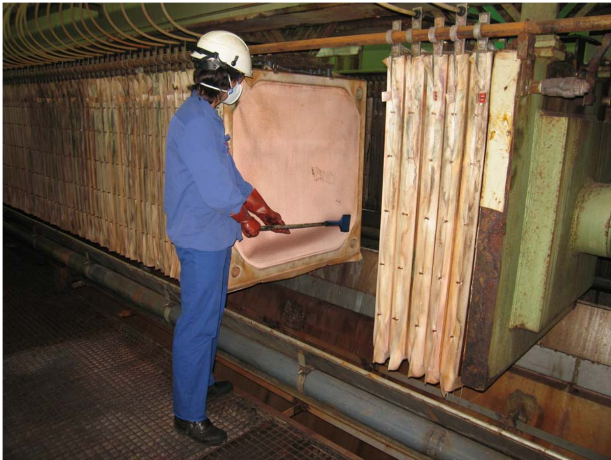
Figure 5. Modified spade with long handle tackles awkward positions
