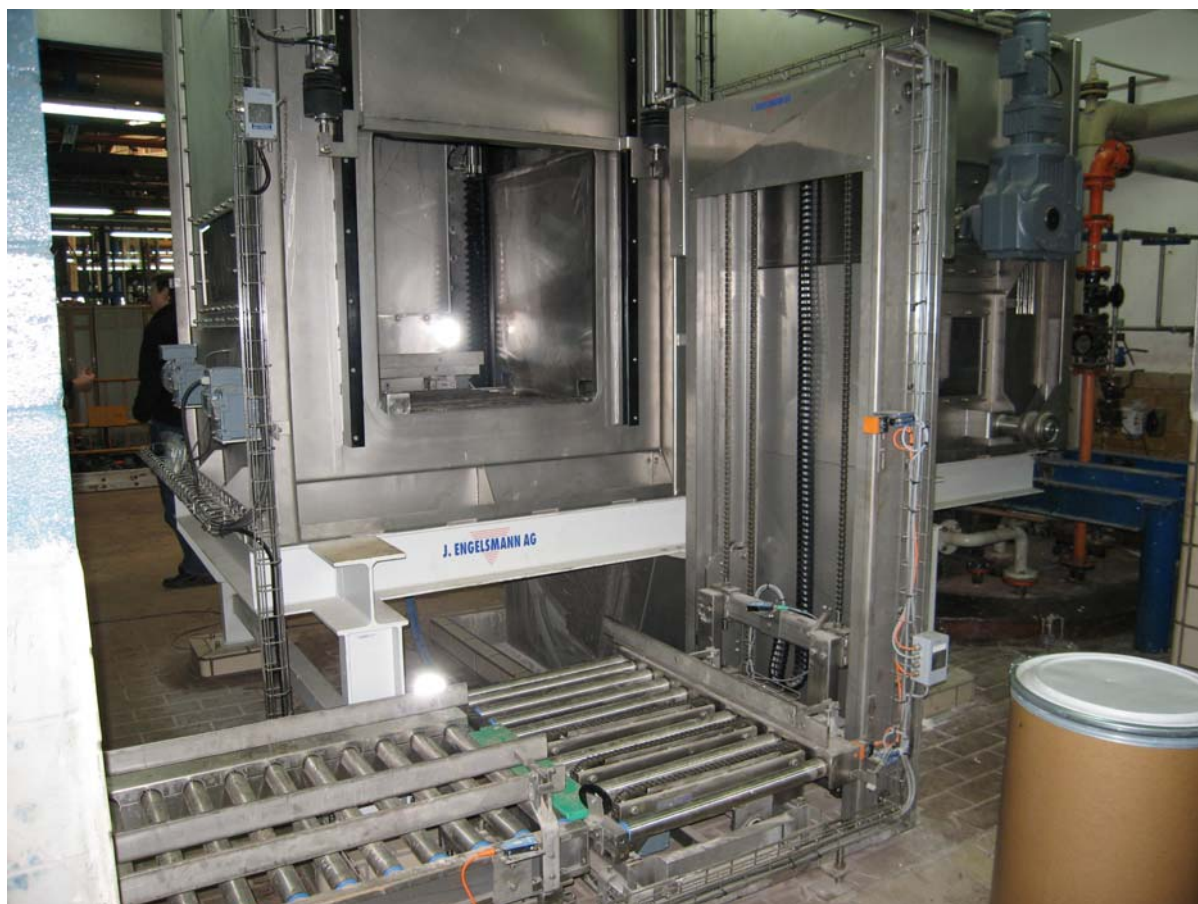
Figure 3. Automatic intake workstation with lift
