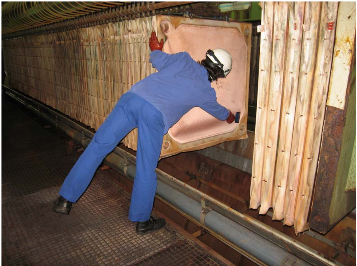
Figure 4. Manual cleaning of filter with the old spade.
