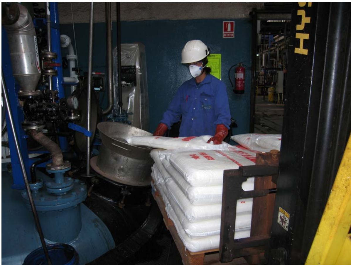
Figure 2. Loading of sacks after intervention: more ergonomic workflow
