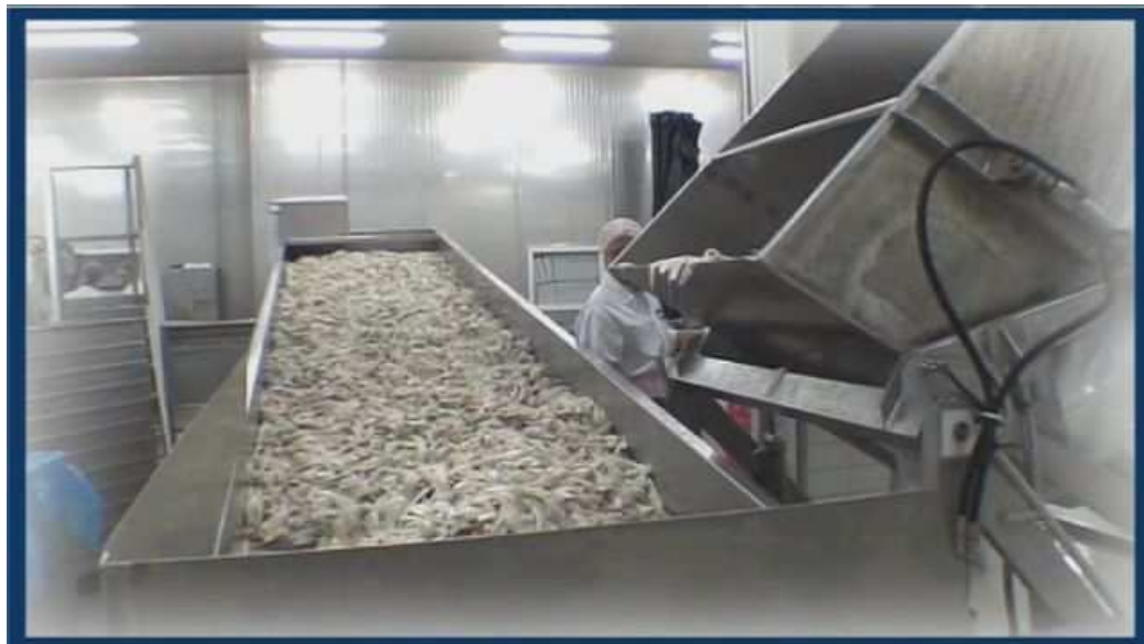
Figure 7. After implementation - the automated draining line transfers the fish to the weighing and packing area and eliminates the need for workers to transport fish using trolleys.
