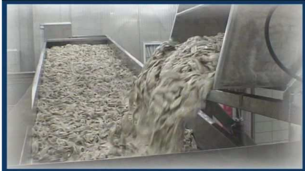
Figure 6. After implementation - the mechanical tipper transfers the contents of the brine container to the automated draining line and eliminates the need to manually pick up fish
