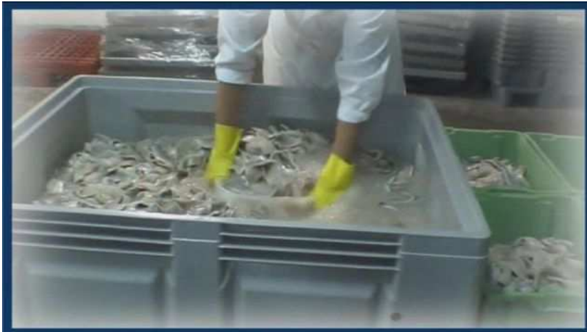
Figure 3: Before improvement – transferring fish via a sieve from the brine container into smaller boxes
