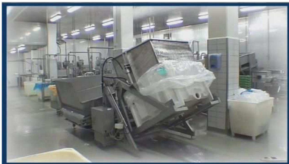
Figure 5. After implementation - the brine container on the mechanical tipper
