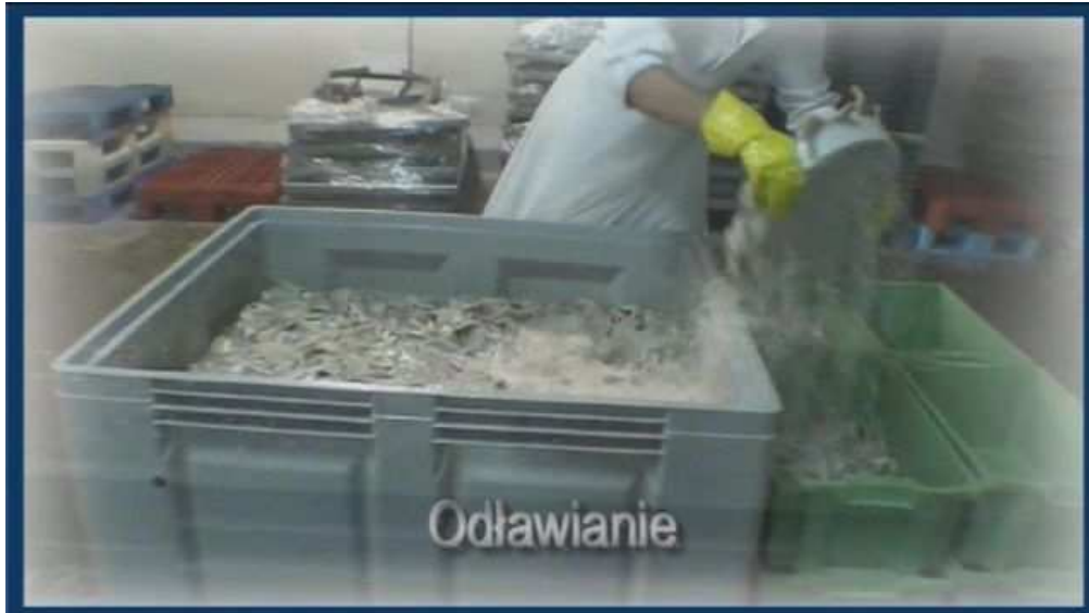
Figure 4. Before implementation of the new solutions, employees were exposed to high musculoskeletal loads, awkward postures and repetitive manual handling
