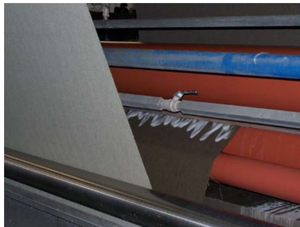
Figure 2: Application of textile finish in a foulard process
