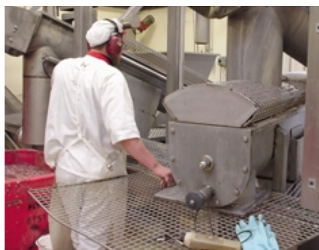
Employee at screw conveyors, which are covered by mesh to prevent accidents. Courtesy of Slagteribranchens Arbejdsmiljøudvalg Slakteri- og Kødbranchens BST, Denmark.
