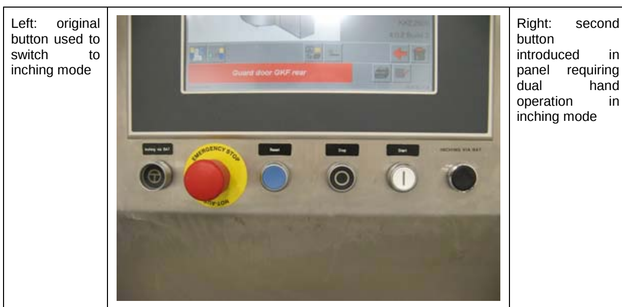
Fig.3 – Detail of improvements made
