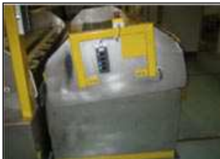
Figure 1. Slitter 13 before modification — risk of crushing fingers
