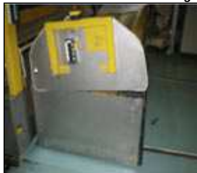
Figure 3. Slitter 13 after modification — risk of crushing fingers has been eliminated
