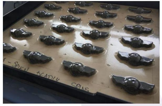
Figure 4. Moulds used in production are made from transparent PET plastic.
