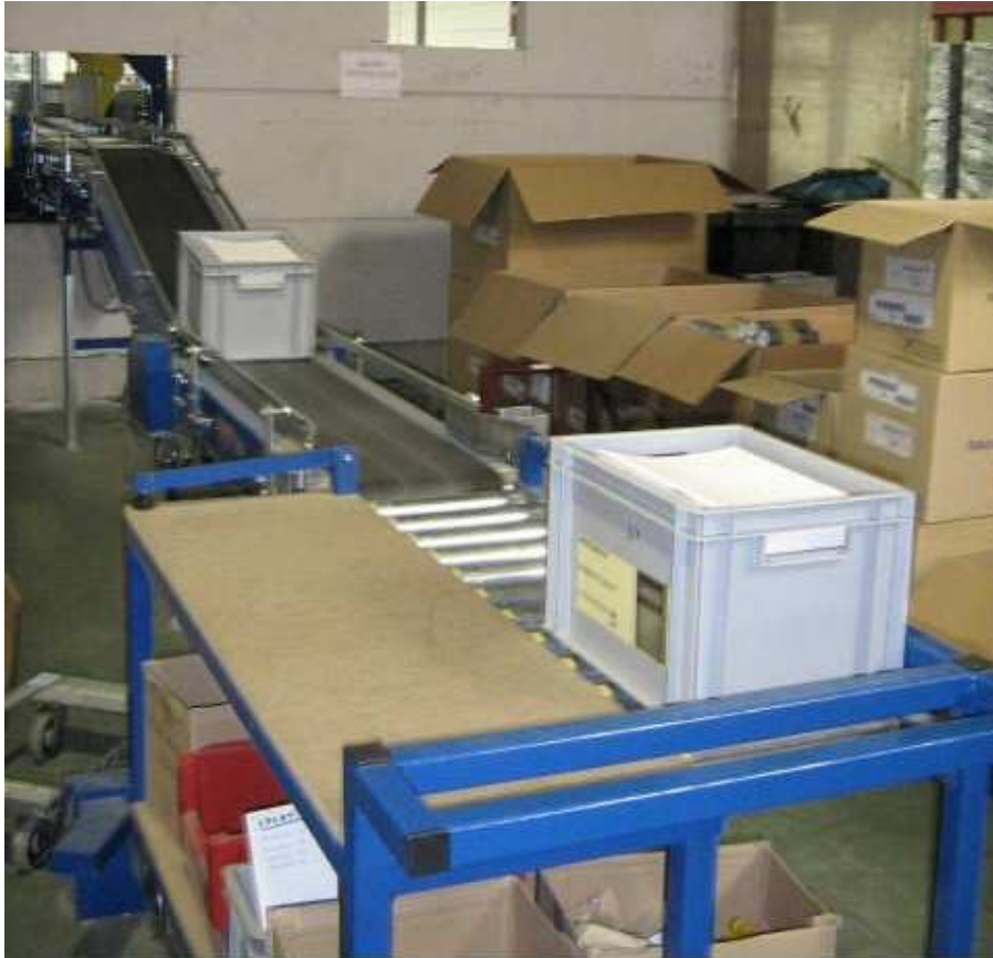
Figure 3 A roller conveyor was introduced for automatic transportation
