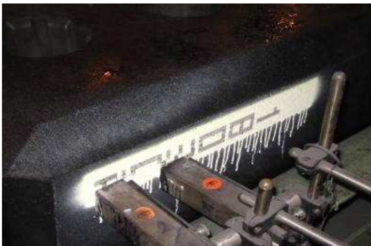
Figure 3 Automated printing device marking the blocks. Photo by Slovalco a.s.
