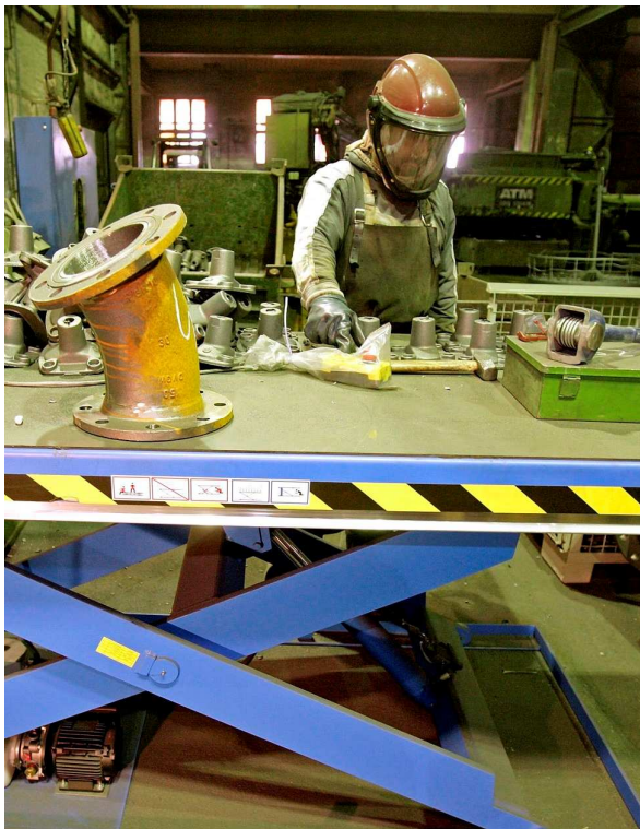
Figure 2 Tipping and lifting tables lighten the load for the workers
