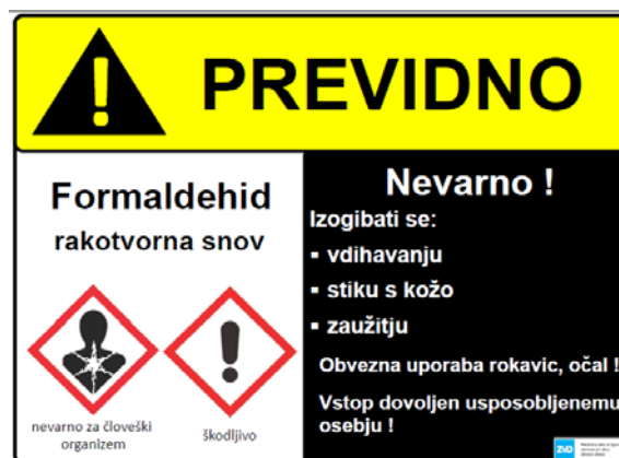
Figure 1. Warning sign with the following safety warnings and instructions: 'Avoid inhalation, contact with skin, ingestion', 'The use of safety gloves and glasses is obligatory', 'Entry is permitted only for trained personnel'.
