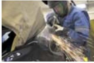
*Before: cross-grinding without the integrated extractor device*
