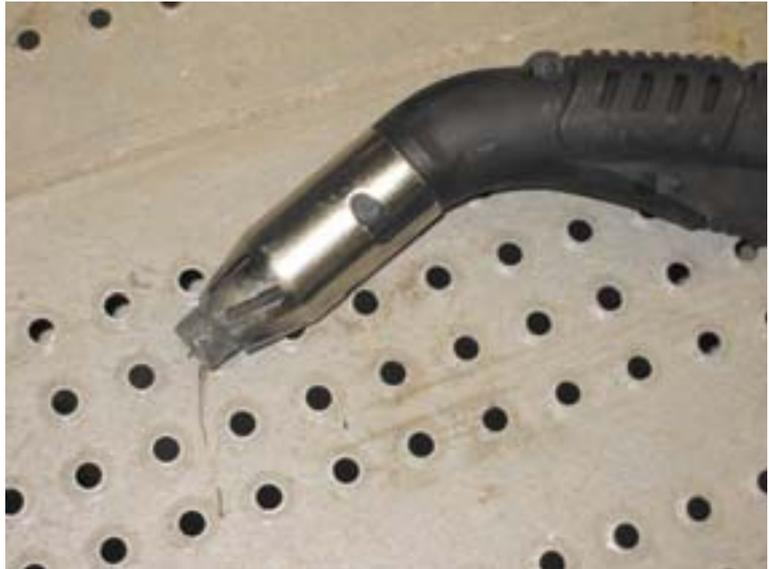
*Integrated extractor fitted to MIG welding gun*
