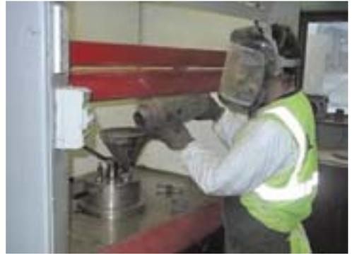
*Old testing method: where a worker pours bitumen and methylene chloride solution into the vacuum pump. The waste methylene chloride was then discharged into a container below the fume cupboard*
