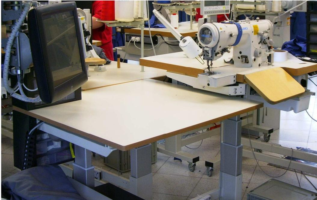
Figure 3 Details of an ergonomic sewing workplace: Arm rests and spacious design help to avoid painful postures
