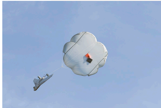
Figure 7: A parachute used to assist the landing of a Eleron-3SV UAV (Wikimedia Commons).
