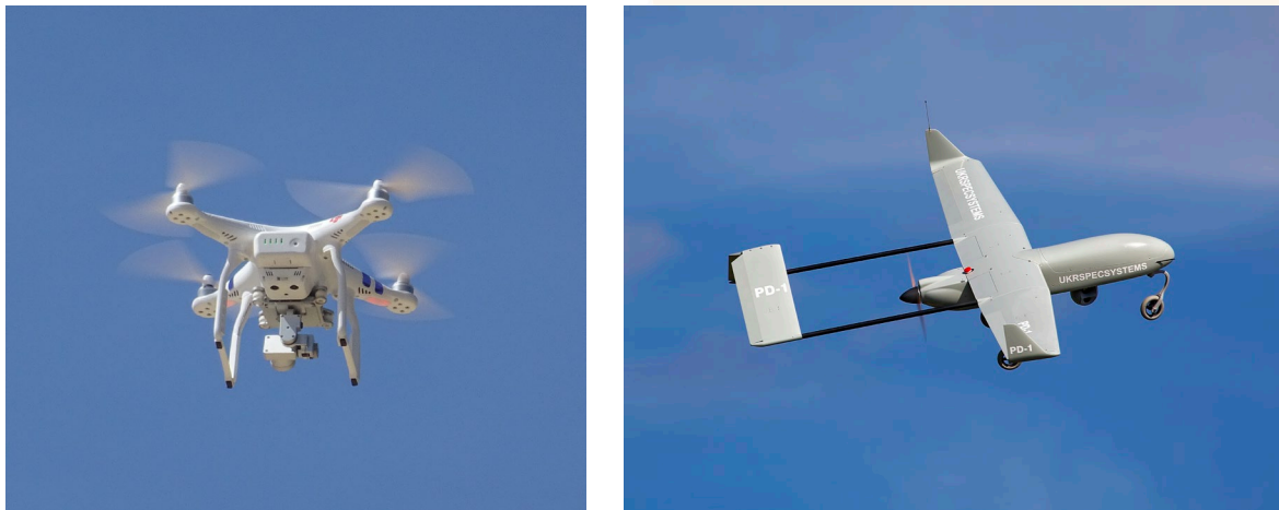
Figure 1: UAV typologies. A four-rotor drone on the left (the load is visible in the underside of the drone – www.publicdomainpictures.net ). A fixed wing UAV is shown in the right image (Wikimedia Commons).
