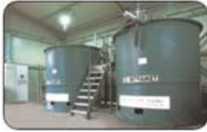
The biological degreasing system
