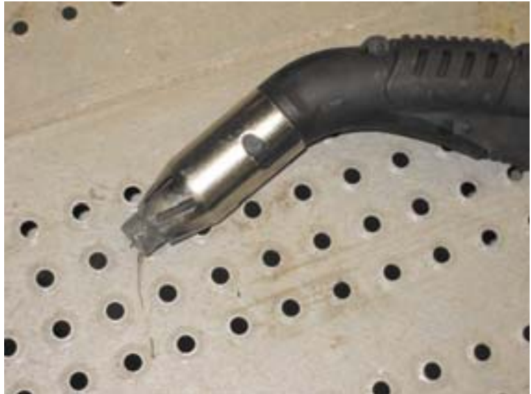
Integrated extractor fitted to MIG welding gun
