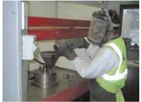
Old testing method: where a worker pours bitumen and methylene chloride solution into the vacuum pump. The waste methylene chloride was then discharged into a container below the fume cupboard
