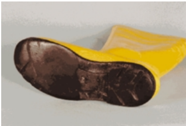
This photo shows a boot that was worn in one of the accidents. It was tested in the laboratory for its anti-slip properties.
