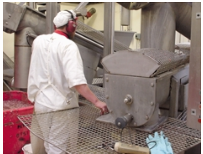
Employee at screw conveyors, which are covered by mesh to prevent accidents. Courtesy of Slagteribranchens Arbejdsmiljøudvalg Slagteri- og Kødbranchens BST, Denmark.
