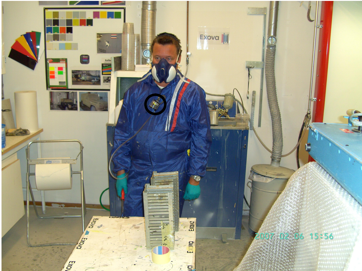
Figure 2: Coating operator with protective clothing. (Measuring device within black circle).
