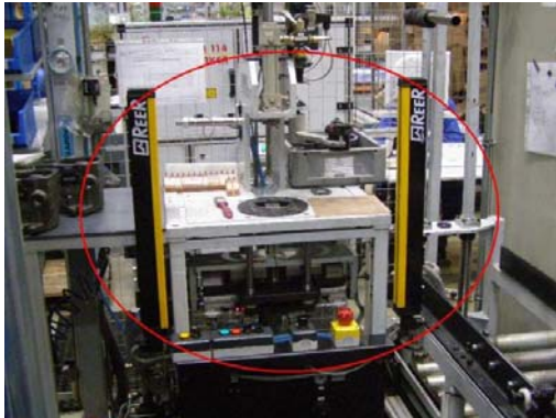
Figure 6. Scan field interruption block the device (press) automatically
