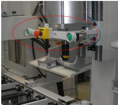
Figure 2. Press with two-handed handling
