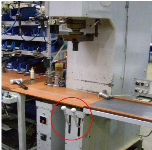
Figure 1. Press with faulty handling
