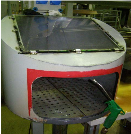
Figure 8. Blowing box protecting the worker from the flying sharp chips at its cleaning process
