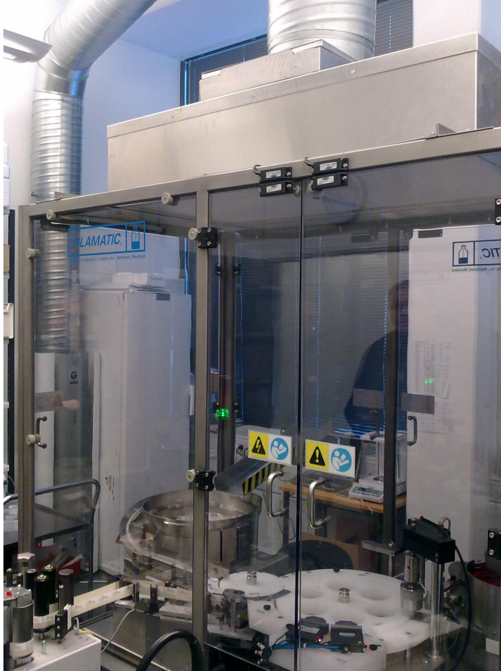
Figure 3: Cabinet of a dispensing machine with pure air connection (on top) from GENANO® air purifier
