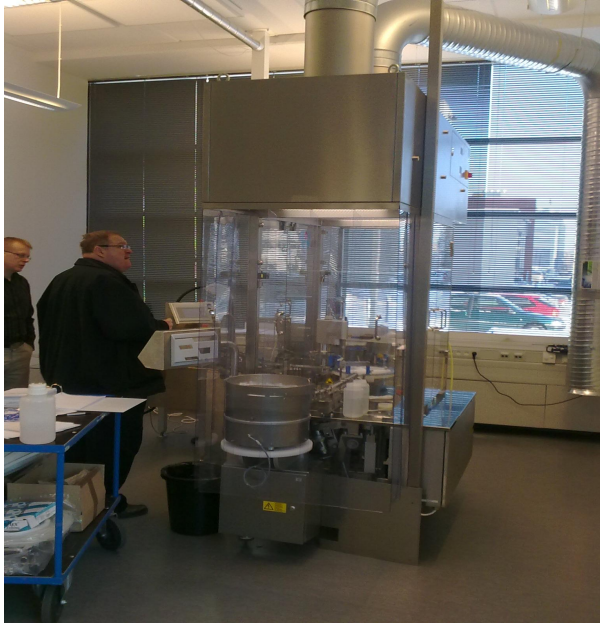
Figure 1: The air purifier is installed and connected to a dispensing machine
